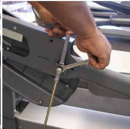
Fig. 6: removing the control link assembly
