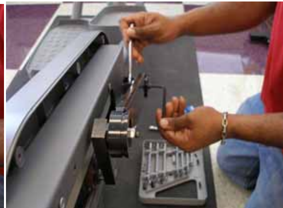
Fig. 8: installing the new control link assembly
